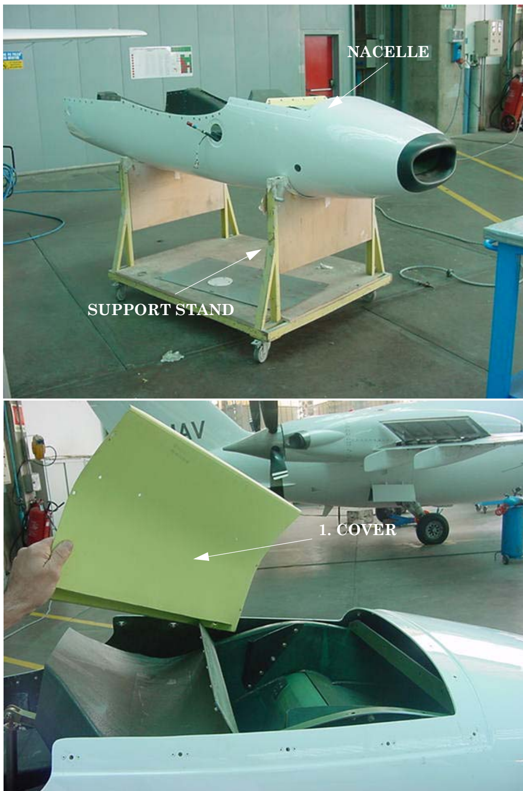
Fig. 203 - Inertial Separator Rear Door - Visual Inspection (Sheet 1 of 3)
